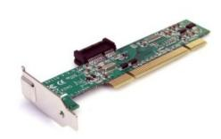
The PCI1PEX1 PCI to PCI Express Adapter card lets you use low profile PCIe expansion cards in a server/desktop motherboard PCI slot. The adapter connects through a 32-bit PCI slot to provide a low profile PCIe x1 slot in its place; a spare, full size bracket is included for installation in larger desktop or server expansion slots that can accommodate a full-sized card.
