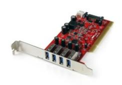
The PCIUSB3S4 4-Port PCI to USB 3.0 Card enables legacy PCI slots to support the SuperSpeed USB 3.0 standard, which is capable of data transfer rates up to 5 Gbps. Using USB 3.0 devices with this card will increase data transfer rates with up to 1.3 Gbps of available bandwidth (PCI bus limit) - more than doubling performance compared to a USB 2.0 connection.
