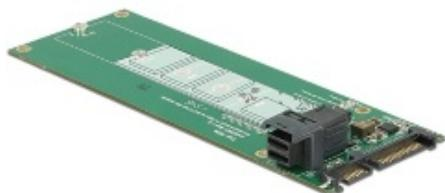
This Delock converter enables the connection of a M.2 NGFF SSD in 2280, 2260, 2242 and 2230 format. It allows the possibility to connect a PCIe or SATA M.2 SSD. The converter can be installed into your system internally through the SATA 22 pin interface while using a SATA M.2 SSD, or via the SFF-8643 interface while using a PCIe M.2 SSD.
