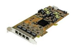
The ST4000PEXPSE 4-Port PoE NIC lets you add four Gigabit Power over Ethernet ports through a single PCI Express slot. Each port can provide up to 25.5W of power, combining network data and power over a single Ethernet cable for reduced cable clutter and added convenience for remote PoE devices.
