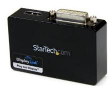
The USB32HDDVII USB 3.0 to HDMI® and DVI-I Dual Head Adapter turns an available USB 3.0 port into one DVI-I or VGA port (DVI to VGA adapter included) and one HDMI® output, with support for high-definition 1080p and 1920x1200 video and 5.1 surround sound audio (from HDMI® port only).
