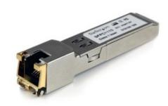
The SFPC1110 Cisco Compatible Gigabit RJ45 Copper SFP Transceiver Module (Mini-GBIC) is built to comply with MSA (Multi-Sourcing Agreement) standards to offer a cost-effective way to add, replace or upgrade a copper Ethernet port on your 1000 Base-T networking equipment.
