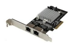
The ST2000SPEXI PCI Express Dual Port Gigabit Network Card lets you add two gigabit Ethernet ports to a desktop computer through a single, four-lane (x4 or higher)PCI Express slot. Each port is fully compatible with IEEE 802.3/u/ab standards, for 10/100/1000 Mbps auto-negotiation.
