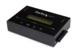
The SATDUP11IMG standalone SATA hard drive duplicator, lets you create an exact duplicate of a SATA hard drive (HDD) / solid state drive (SSD), or create a single backup library drive containing multiple images you can copy to additional drives at any time.
