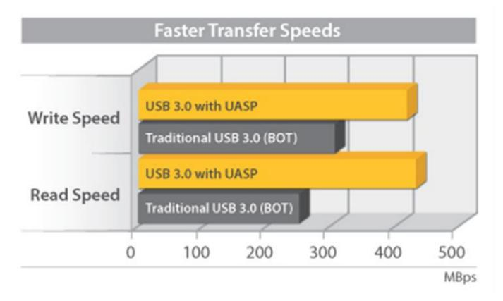
At the same peak in testing, UASP also showed up to an 80% reduction in required processor resources.
